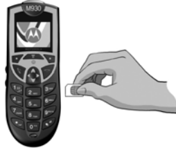
Figure 2. Inserting the SIM card into the phone.
